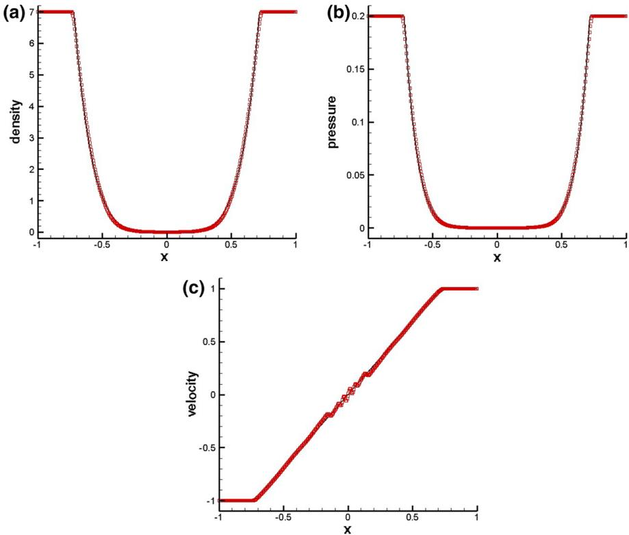
**Fig. 3** Double rarefaction.  $T=0.6$ . Cut at  $y = 0$ .  $\Delta x = 1/200$ . HWENO scheme with the positive-preserving limiter. The *solid line* is the exact solution. *Symbols* are numerical solutions
