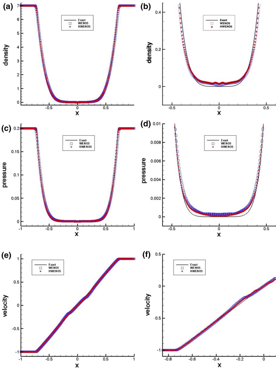
**Fig. 2** Double rarefaction.  $T=0.6$ . *left* 1D problem. *Right* the zoom.  $\Delta x = 1/200$ . HWENO5 and WENO5. The *solid line* is the exact solution. *Squares* numerical solution of WENO5; *Pluses* numerical solution of HWENO5
