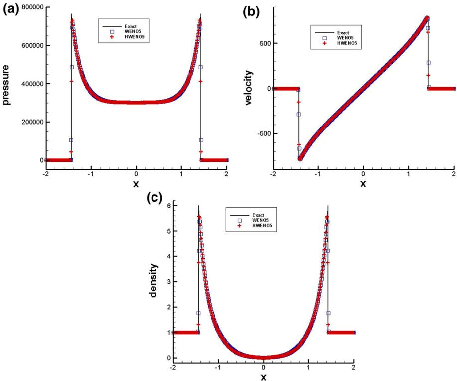
**Fig. 1** 1D Sedov blast.  $T=0.001$ .  $\Delta x = 0.01$ . HWENO5 and WENO5. The solid line is the exact solution. Squares numerical solution of WENO5; Pluses numerical solution of HWENO5
