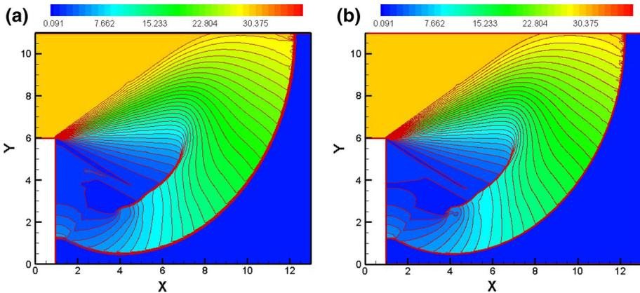
**Fig. 5** Shock diffraction problem.  $T = 2.3$ . Pressure, 40 equally spaced contour lines from  $p = 0.091$  to  $p = 37$
