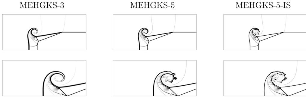
Fig. 7. The schlieren-type images of  $\rho$  of the triple point problem with  $840 \times 360$  cells at  $t = 2.4$  (top) and  $t = 5$  (bottom).
