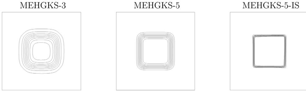
Fig. 5. The contours of  $\rho$  of the two-dimensional square wave propagating problem with  $80 \times 80$  cells at  $t = 4$ .
