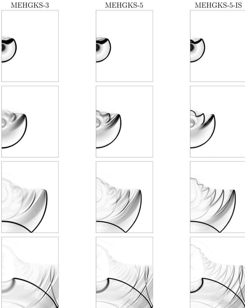
Fig. 11. The schlieren-type images of  $p$  of the underwater explosion problem with  $400 \times 500$  cells at  $t = 2 \times 10^{-4}, 4 \times 10^{-3}, 8 \times 10^{-3}$  and  $1.2 \times 10^{-3}$  (from top to bottom).
